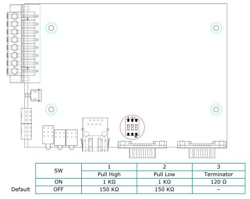
In some critical environments, you may need to add termination resistors to prevent the reflection of serial signals. When using termination resistors, it is important to set the pull high/low resistors correctly so that the electrical signal is not corrupted. The MGate uses jumper settings or DIP switches to set the pull high/low resistor values for each serial port.
