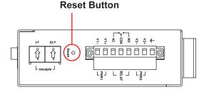
To reset the MGate to the factory default settings, hold down the reset button for about 5 seconds. The MGate will restart and be reset to factory default settings.
