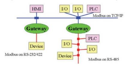
Ordinarily, Modbus TCP and Modbus ASCII/RTU cannot communicate with each other.
