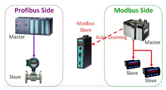
After some time, MGate 4101-MB-PBS will fully learn the requests from the Modbus client/master. Through this QuickLink process, the MGate 4101-MB-PBS can replace the legacy Modbus client/master. Moreover, the MGate 4101-MB-PBS can respond to all the Modbus servers/slaves correctly.
