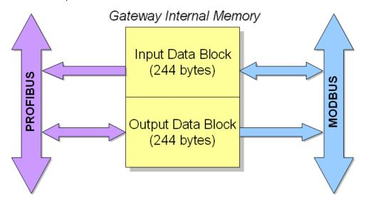
Input refers to the dataflow from the Modbus device to the PROFIBUS master. It means the gateway will read the Modbus device's data and store in its input memory area. And the PROFIBUS master will read these Modbus data stored at the gateway's input memory. Users can choose an internal memory address between 0 to 224.
