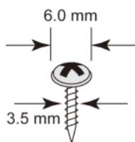
**NOTE** Before tightening the screws into the wall, make sure the screw head and shank size are suitable by inserting the screw through one of the keyhole-shaped apertures of the Wall Mounting Plates.
