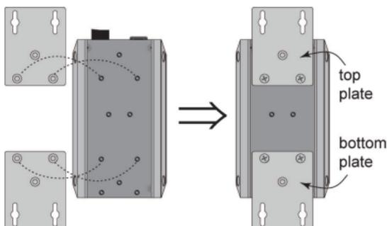
**STEP 2**—Mounting the EDS-G512E-8PoE series on the wall requires 4 screws. Use the EDS-G512E-8PoE series, with wall mount plates attached, as a guide to mark the correct locations of the 4 screws. The heads of the screws should be less than 6.0 mm in diameter, and the shafts should be less than 3.5 mm in diameter, as shown in the figure on at right.
