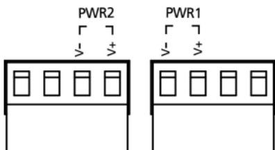
**STEP 1:** Insert the negative/positive DC wires into the V-/V+ terminals, respectively.
