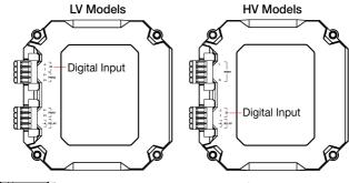
**STEP 1:** Insert the negative (ground)/positive DI wires into the -I/I terminals, respectively.
