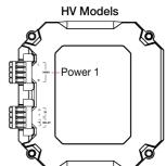
**STEP 1:** Insert the Positive/Negative DC or Line/Neutral AC wires into the V+/V- or L/N terminals, respectively.
