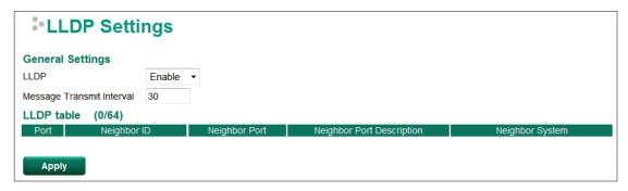
The router's web interface can be used to enable or disable LLDP, and to set the LLDP **Message Transmit Interval**. Users can view each switch's neighbor-list, which is reported by its network neighbors.
