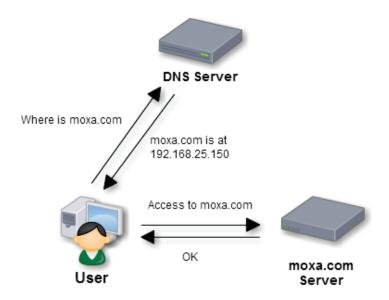
From the Global Settings screen, you can configure basic DNS server functions such as the server type and service interfaces. If **Recursive** mode is selected, a built-in root hints file will be applied by default. However, user can still configure up to 2 additional user-defined root servers. If there is a conflict between the FQDNs of user-defined servers and those in the root hints file, user-defined servers have higher priority and will be adopted first.
