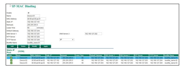
In the above example, a device named "Device-01" was added to the Static DHCP list, with a static IP address set to 192.168.127.101 and MAC address set to 00:09:ad:00:aa:01. When a device with a MAC address of 00:09:ad:00:aa:01 is connected to the ToughNet Secure Router, the ToughNet Secure Router will offer the IP address 192.168.127.101 to this device.
