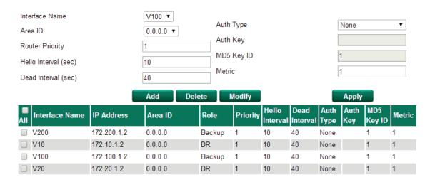
Before using OSPF, you need to assign an interface for each area. Detailed information related to the interface can be defined in this section.
