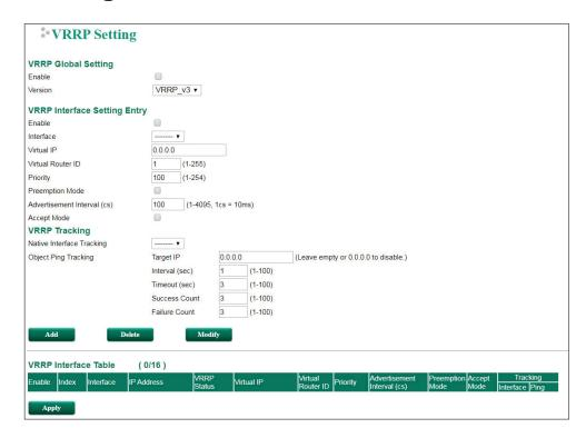
Virtual Router Redundancy Protocol (VRRP) can solve the problem with static configuration. VRRP enables a group of routers to form a single virtual router with a virtual IP address. The LAN clients can then be configured with the virtual router's virtual IP address as their default gateway. The virtual router is the combination of a group of routers, and is also known as a VRRP group.
