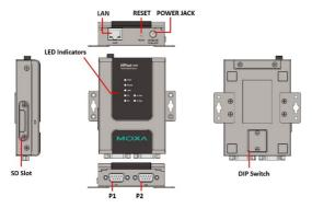
**Reset Button**—Press the Reset Button continuously for 5 sec to load factory defaults. Use a pointed object, such as a straightened paper clip or toothpick, to press the reset button. This will cause the Ready LED to blink on and off. The factory defaults will be loaded once the Ready LED stops blinking (after about 5 seconds). At this point, you should release the reset button.
