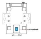
Open the back door with a screwdriver and use the DIP switch to set the pull high/low resistors. The default is 150 k $\Omega$ . You can switch the SW1 and SW2 to ON and change the resistors value to 1 k $\Omega$ .
