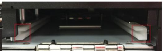
6. Insert the tray so that it aligns with the rails on both sides and slide the tray into the slot.
