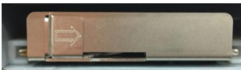
To take out the tray, simply pull the clutch to the right and pull the tray out.
