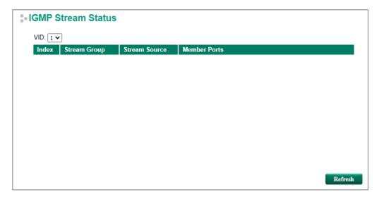
**Stream Group:** Multicast group IP address **Stream Source:** Multicast source IP address
