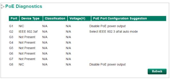
**PoE Diagnose** helps users determine the PD conditions. The system provides the user with configuration options; select the best option for your PDs. Take the following steps to diagnose PD conditions:
