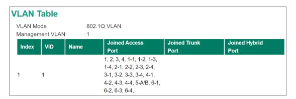
Use the 802.1Q VLAN table to review the VLAN groups that were created, VLAN Name, Joined Access Ports, Trunk Ports, and Hybrid Ports.
