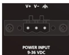
Connect the power connector/terminal block to the power supply that can provide 9 to 36 VDC (MC-3201-TGL1 model) or 24 VDC (MC-3201-TGL7 model). Before connecting the device to DC power inputs, make sure the DC power source voltage is stable. If the power is supplied properly, the Power LED will light up. The OS is ready when the Power LED glows solid green.
