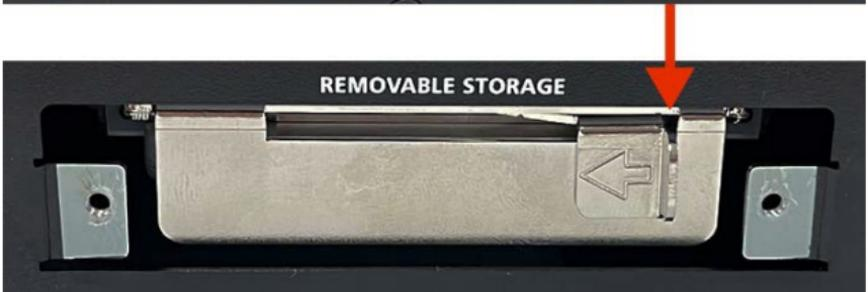
**Step 7:** Put back the cover on the storage slot and fasten the two screws to secure the cover in place.
