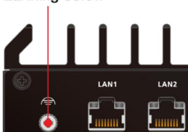
**NOTE** A 4 mm<sup>2</sup> conductor must be used when the connection to the external grounding screw is utilized. The heat sink is grounded to the chassis by an internal screw.
