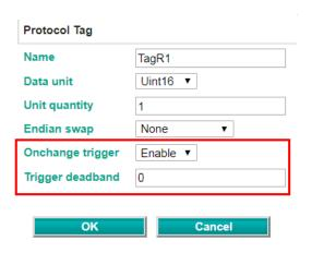
So when the MGate 5105 gets Modbus RTU device Register0's value changed, it triggers to publish message to AWS IoT Thing.
