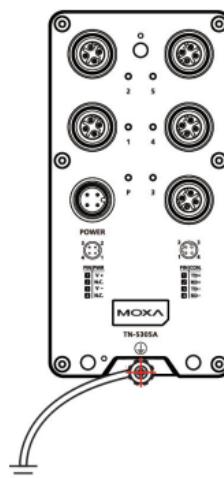
**STEP 1:** Connect the grounding wire (AWG 22 or larger) to the grounding screw and connect the other end of the wire to ground.
