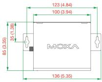
The mounting kit is 2 mm in height, and the two centers of the mounting kit on each plate is 163 mm (UPort 207A) and 123 mm (UPort 204A) apart.
