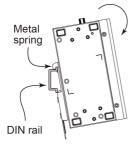
**STEP 2:** Press the UPort<sup>™</sup> 200A towards the mounting rail until it snaps into place.
