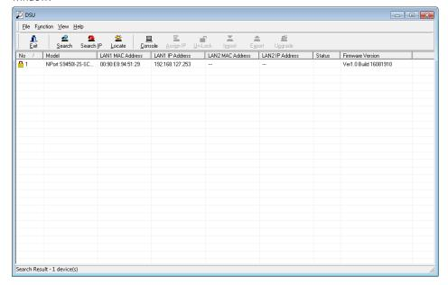
3. To modify the configuration of the highlighted NPort S9000, click on the Console icon to open the web console. This will take you to the web console, where you can make all configuration changes. Please refer to Chapter 6, "Configuration with the Web Console", for information on how to use the web console.
