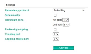
**NOTE** The user does not need to set the master to use Turbo Ring. If no master is set, the Turbo Ring protocol will assign master status to one of the NPort S9000 in the ring. The master is only used to determine which segment serves as the backup path.
