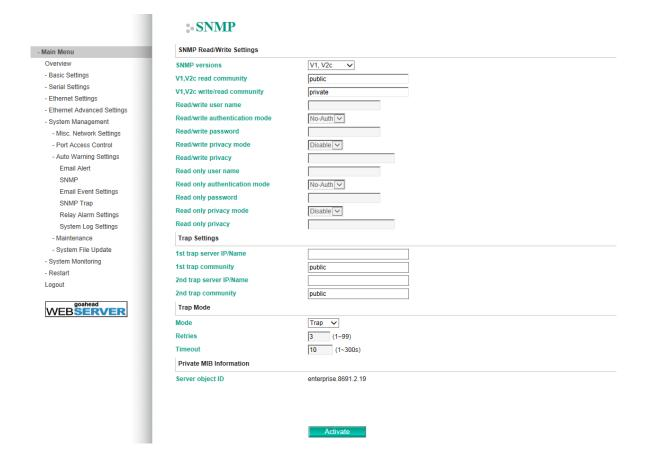
**SNMP agent version:** The NPort S9000 supports SNMP V1, V2c, and V3.
