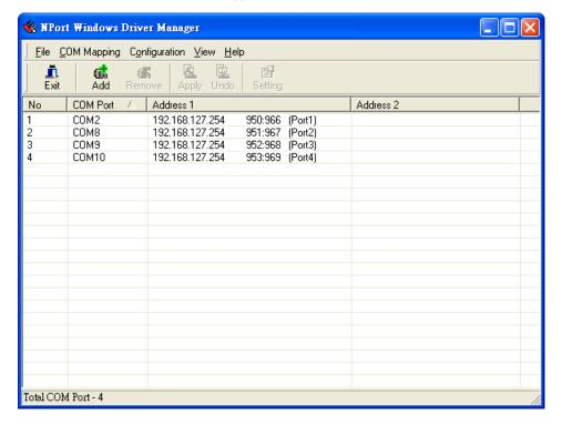
8. Use terminal software to open the mapped COM port to communicate with the serial device. You may download PComm Lite, a useful tool to check the serial communication, from Moxa's website: <a href="http://www.moxa.com/support/download.aspx?type=support&id=167">http://www.moxa.com/support/download.aspx?type=support&id=167</a>
