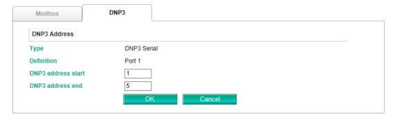
When you select a serial routing and click **Edit**, you can assign the configuration for DNP3 packet frames coming from the serial side and will need to assign the DNP3 slave IDs.
