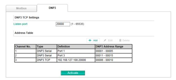
The gateway will drop a DNP3 packet frame if the destination DNP3 device address or IP address is not defined in the gateway.
