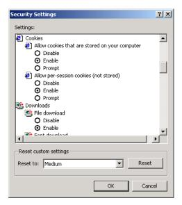
2. After using the DSU to find a specific NPort, type the IP address to log in to the web console. If this is the first time you configure the NPort, you may directly type the default IP address, 192.168.127.254 in the Address input box. Use the correct IP address if it is different from the default and then press Enter.
