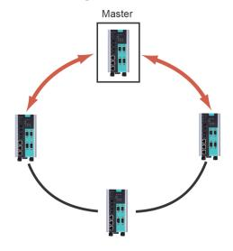
For a "Turbo Ring V2" ring, the backup segment is the segment connected to the second redundant port on the master.
