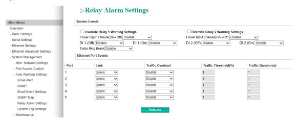
Event Types can be divided into two basic groups: **System Events** and **Ethernet Port Events**. System Events are related to the overall function of the NPort S9000, whereas Ethernet Port Events are related to the activity of a specific port.
