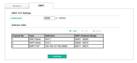
When you click **Add**, you can add the master (or outstation) devices on the Ethernet side. You will need to add these devices' IP address and DNP3 address to the routing table.
