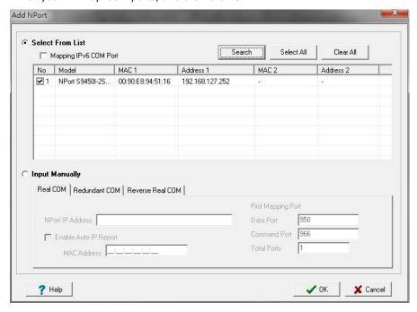
4. Alternatively, you can select **Input Manually** and then manually enter the NPort IP Address, 1st Data Port, 1st Command Port, and Total Ports to which COM ports will be mapped. Click **OK** to proceed to the next step. Note that the Add NPort page supports FQDN (Fully Qualified Domain Name), in which case the IP address will be filled in automatically.
