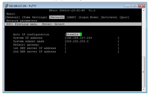
8. Press **Esc** to return to the previous page. Select **Activate** and press **Y** to confirm the modification and activate the new settings.
