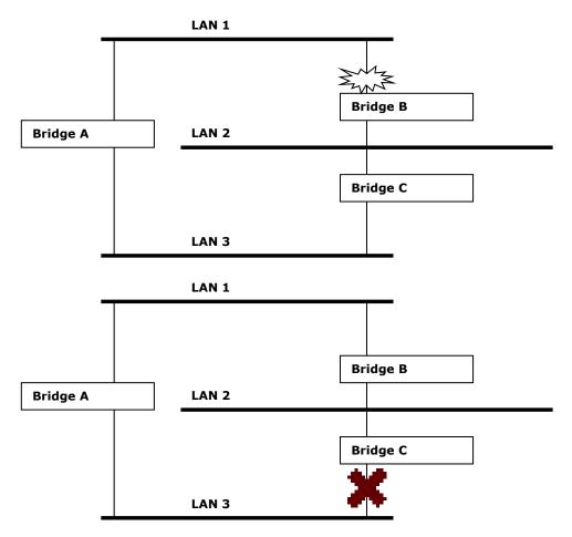
What happens if a link failure is detected? As shown in the previous figure, the STP process reconfigures the network so that traffic from LAN segment 2 flows through Bridge B.
