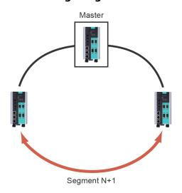
If there are 2N+1 NPort S9000 (an odd number) in the "Turbo Ring" ring, with the NPort S9000 and segments labeled counterclockwise, then segment N+1 will serve as the backup path.
