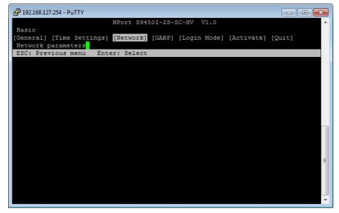
7. Use the arrow keys to move the cursor to System IP address. Use the **Delete**, **Backspace**, or **Space** key to erase the current IP address, and then type in the new IP address and press **Enter**. If you are using a dynamic IP configuration (BOOTP or DHCP), you will need to go to the Auto IP configuration field and press **Enter** to select the appropriate configuration.
