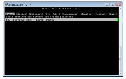
6. Press **N**, or use the arrow keys to select network and then press **ENTER** to configure Network parameters.
