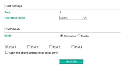
Outstation and master devices have a logical device address for identification in the DNP3 system. You need to set the address table to indicate the routing destination of the DNP3 packet frames received by the gateway. Please go to Serial Settings --> Protocol Settings under the DNP3 tab for relative settings. A default device address routing table is shown in the Address table page under Protocol Settings.
