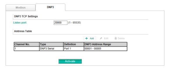
For the DNP3 TCP Settings, you may modify which TCP port should the device server listen to for DNP3 packet frames. The default port is 20000.For the Address Table, you may Add/Edit/Delete for the device address routing table.
