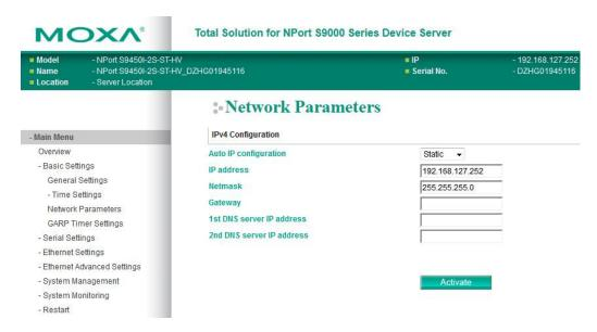
You must assign a valid IP address to the NPort S9000 before it will work in your network environment. Your network system administrator should provide you with an IP address and related settings for your network. The IP address must be unique within the network; otherwise, the NPort S9000 will not have a valid connection to the network. First-time users can refer to Chapter 3, "Initial IP Address Configuration," for more information.
