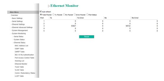
This page illustrates the data transmission status of Ethernet. Check one of the four options, Total Packets, TX Packets, RX Packets, or Error Packets, to show the transmission activity of specific types of packets.
