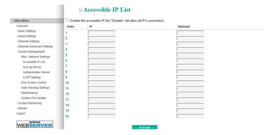
Accessible IP Settings allows you to add or remove "Legal" remote host IP addresses to prevent unauthorized access. Access to the NPort S9000 is controlled by an IP address. If a host's IP address is in the accessible IP table, then the host will be allowed access to the NPort S9000. You can allow one of the following cases by setting this parameter:
