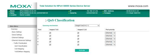
The NPort S9000 supports inspection of layer 3 TOS and/or layer 2 CoS tag information to determine how to classify traffic packets.
