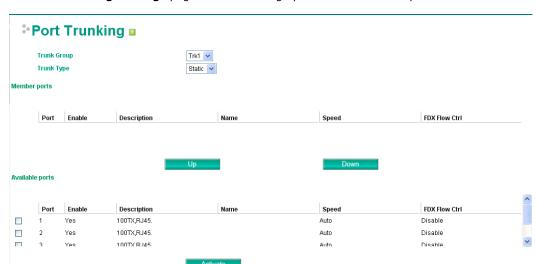
The **Port Trunking Settings** page is used to assign ports to a Trunk Group.
