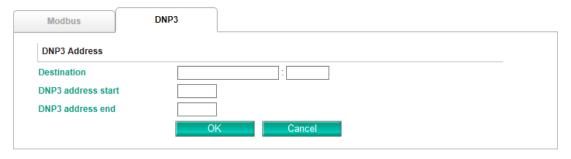
When you click Add, you can add the master (or outstation) devices on the Ethernet side. You will need to add these devices' IP address and DNP3 address to the routing table.
