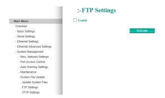
The NPort S9000 can be a FTP server to save configuration file or log files on it. You may enable it by checking the checkbox **Enable** and then click **Activate**.
