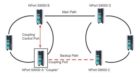
To configure the Ring Coupling function for a "Turbo Ring" ring, select two NPort S9000 devices (e.g., Device A and B in the above figure) in the ring, and another two NPort S9000 devivces in the adjacent ring (e.g., Device C and D).
