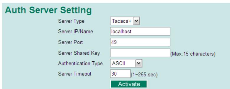
The screenshot shows the 'Auth Server Setting' interface for TACACS+. It includes the following fields: Server Type (Tacacs+), Server IP/Name (localhost), Server Port (49), Server Shared Key (empty, with a note '(Max. 15 characters)'), Authentication Type (ASCII), and Server Timeout (30, with a note '(1~255 sec)'). A green 'Activate' button is at the bottom.
