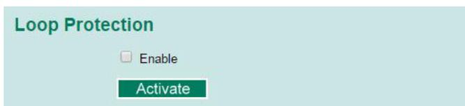
Check the Enable box and click Activate to enable the Loop protection.
