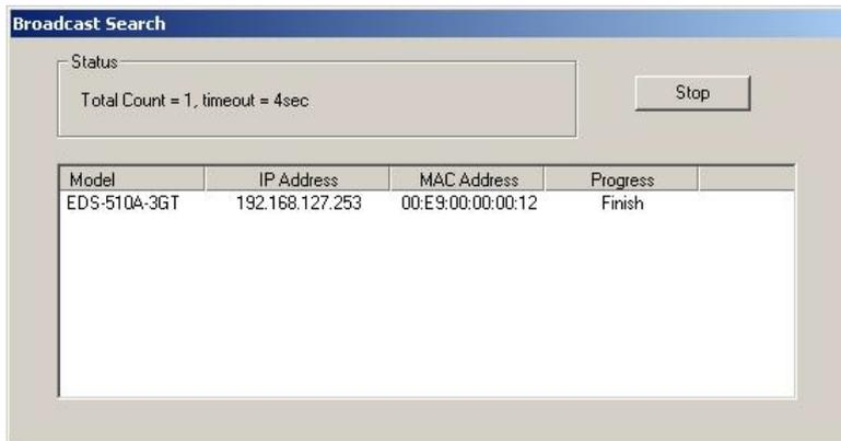
2. Once the search is complete, the Configurator window will display a list of all switches that were located.
