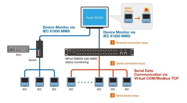
Serial device servers with MMS, on the other hand, allow substation engineers to manage all networking devices under one software view. They do not only provide the status of networking equipment but also update the status of serial communication. This is beneficial because before sending any field engineer to a distant location, one can determine where the fault might be by clarifying whether it is a:
