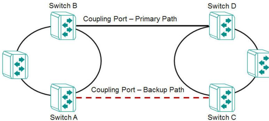
For Turbo Ring V2, Ring Coupling is enabled by configuring the **Coupling Port (Primary)** on Switch B, and the **Coupling Port (Backup)** on Switch A only.
