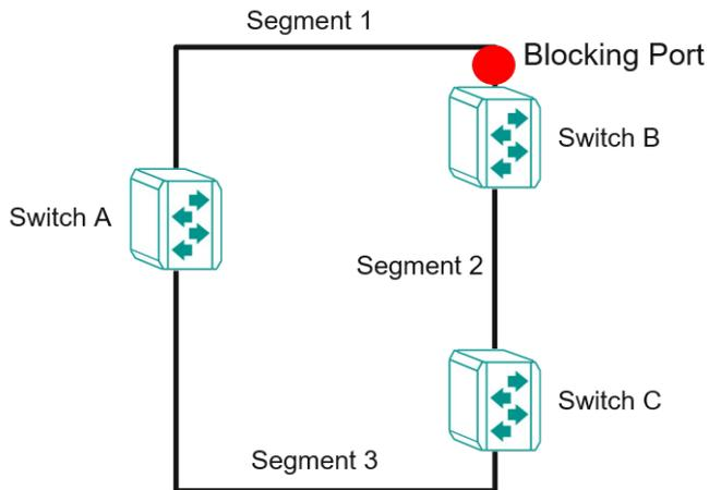
What happens if a link failure is detected? As shown in the figure below, the STP will change the blocking state to a forwarding state so that traffic from segment 2 flows through switch B to segment 1 through a redundant path.
