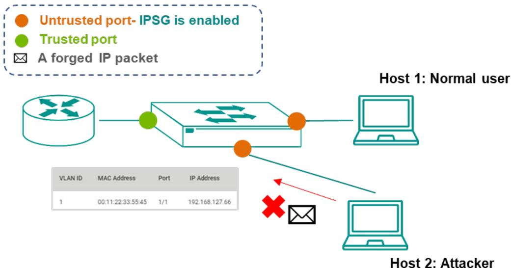
Click **IP Source Guard** on the function menu to enable the feature by individual ports or copy configurations to multiple ports. Please note IPSG can only be enabled on untrusted ports specified in DHCP Snooping feature. Click the
