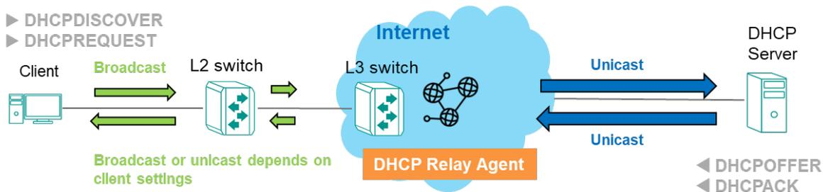
When the DHCP Relay Agent is set on an L2 switch, the switch would convert the broadcast packets to unicast packets and forward them to the L3 switch to route to the DHCP server.
