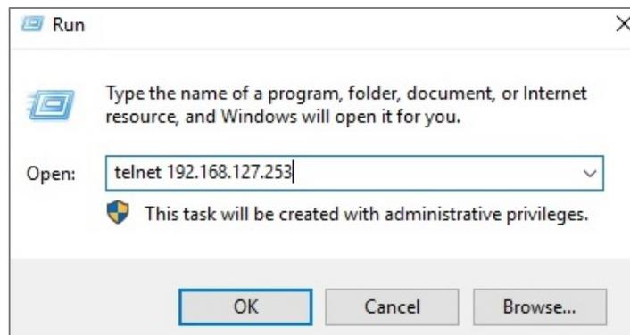
12. The Telnet console will prompt you to log in. The default login name is **admin**, and the password is **moxa**. This password will be required to access any of the consoles (web, serial, Telnet).
