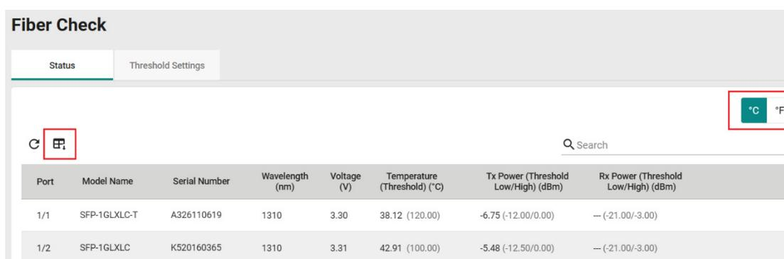
The screenshot shows the 'Fiber Check' web interface. At the top, there are two tabs: 'Status' (selected) and 'Threshold Settings'. Below the tabs, there is a temperature unit selector with '°C' and '°F' icons. A search bar is also present. The main content is a table with the following data:
