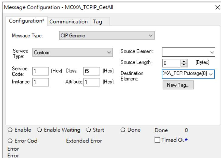
Click the Communication tab and set up the communication path to the Moxa Ethernet switch for **Get\_TCPIP\_AllMessage**.
