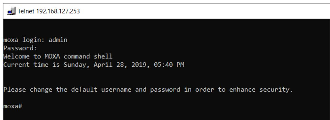
13. After successfully connecting to the switch by Telnet, users can start configuring the switch parameters by using command line instructions. Refer to the **Moxa Command Line Interface Manual**.
