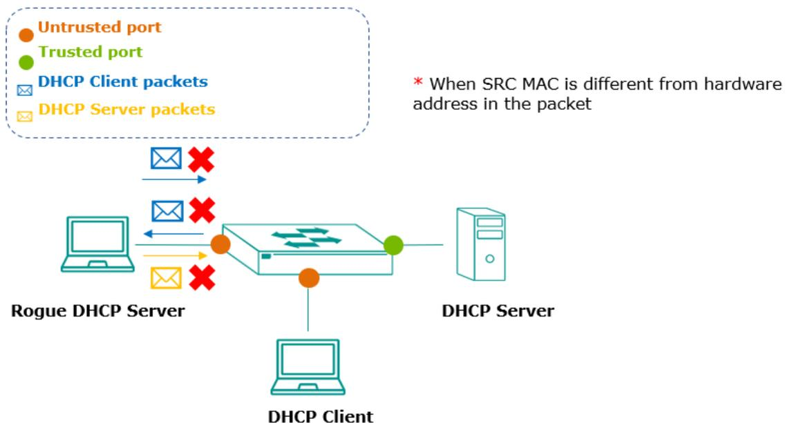
The successful DHCP transaction with DHCP Snooping enabled will create and update the Binding Database. Binding Database contains VLAN ID, MAC Address, untrusted port of DHCP clients and IP Address. Binding Database can also be used for other security functions, such as IP Source Guard and Dynamic ARP Inspection.
