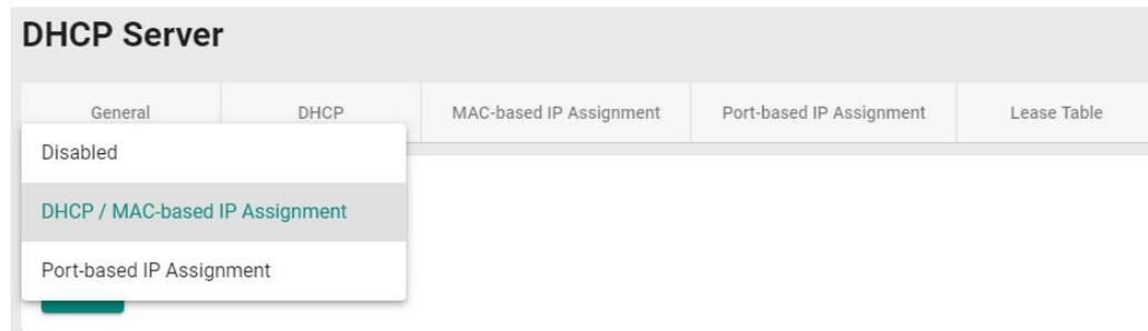
The screenshot shows the 'DHCP Server' configuration page with the 'General' tab selected. A dropdown menu is open, showing three options: 'Disabled', 'DHCP / MAC-based IP Assignment' (which is highlighted in blue), and 'Port-based IP Assignment'.
