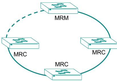
One ring port of the MRM shall be connected to a ring port of an MRC. The other ring port of that MRC shall be connected to a ring port of another MRC or to the second ring port of the MRM.
