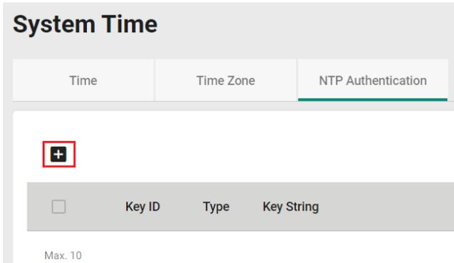
The screenshot shows the 'System Time' configuration page with the 'NTP Authentication' tab selected. A table is visible with columns for 'Key ID', 'Type', and 'Key String'. A red box highlights a plus icon in the top-left corner of the table area. Below the table, it says 'Max. 10'.
