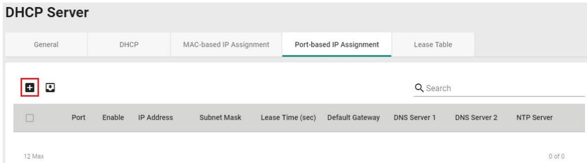
The screenshot shows the 'DHCP Server' configuration page with the 'Port-based IP Assignment' tab selected. A table is visible with a search bar and a '+ Add' icon. The table has columns for 'Port', 'Enable', 'IP Address', 'Subnet Mask', 'Lease Time (sec)', 'Default Gateway', 'DNS Server 1', 'DNS Server 2', and 'NTP Server'. The table is currently empty, showing '12 Max' and '0 of 0' entries.
