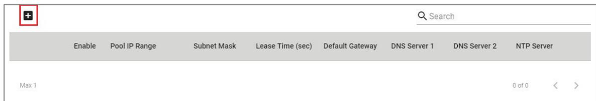
The screenshot shows the DHCP configuration page with a table of DHCP server pools. The table has columns for 'Enable', 'Pool IP Range', 'Subnet Mask', 'Lease Time (sec)', 'Default Gateway', 'DNS Server 1', 'DNS Server 2', and 'NTP Server'. A red box highlights the '+' icon in the top left corner of the table area. The table is currently empty, showing 'Max 1' and '0 of 0'.
