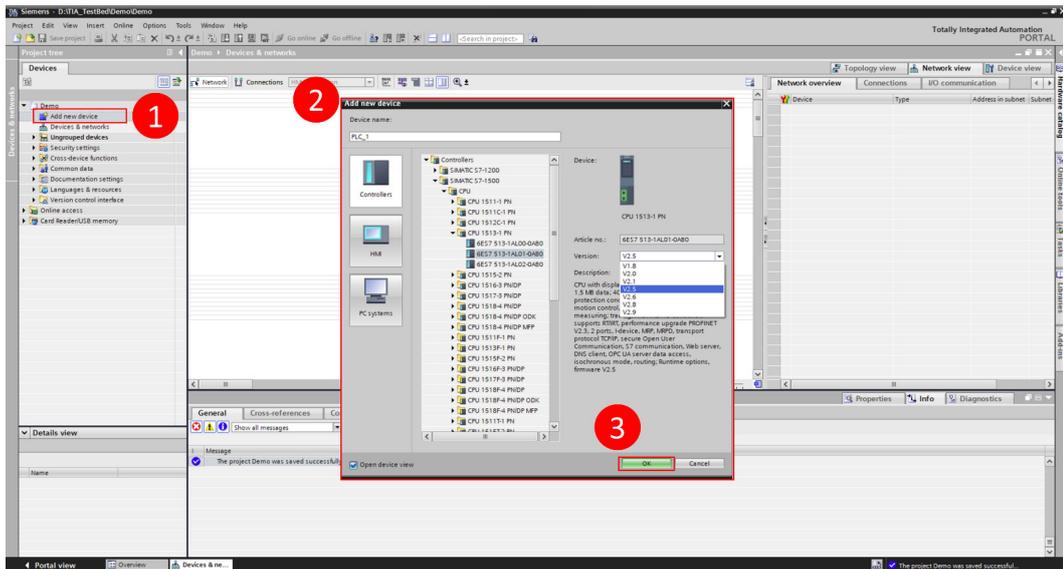
4. In the **Devices** tab, click **Device & networks** and select the switch you want to add from the **Hardware catalog** section.
