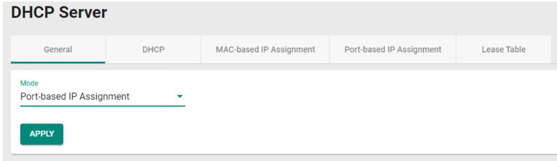
The screenshot shows the 'DHCP Server' configuration page with the 'General' tab selected. The 'Mode' dropdown menu is set to 'Port-based IP Assignment'. A green 'APPLY' button is visible at the bottom left of the configuration area.
