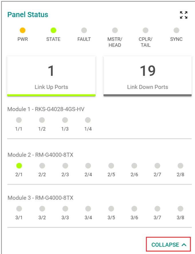
The expanded Panel Status view shows detailed port status for three modules. Module 1 (RKS-G4028-4GS-HV) has 4 ports (1/1 to 1/4), all gray. Module 2 (RM-G4000-8TX) has 8 ports (2/1 to 2/8), with 2/1 green and others gray. Module 3 (RM-G4000-8TX) has 8 ports (3/1 to 3/8), all gray. A red box highlights the collapse icon in the top right corner. A COLLAPSE button with an upward arrow is located at the bottom right.
