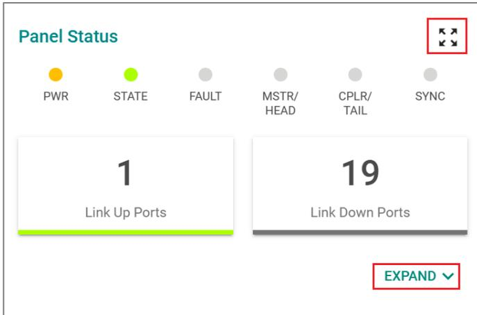
The Panel Status summary view displays several indicators: PWR (yellow dot), STATE (green dot), FAULT (gray dot), MSTR/HEAD (gray dot), CPLR/TAIL (gray dot), and SYNC (gray dot). It shows 1 Link Up Port and 19 Link Down Ports. A red box highlights the expand/collapse icon in the top right corner. An EXPAND button with a downward arrow is located at the bottom right.
