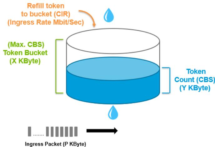
**CAR (Committed Access Rate)** is a traffic control mechanism used to ensure that packets meet the network rules before they enter the network. CAR can guarantee the traffic flow is under user-defined control; the packets exceeding the rule will be either dropped or remarked and transmitted again. When network traffic is jammed, these packets will be dropped first.
