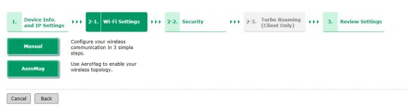
For additional details on the AeroMag function, refer to the *Wireless LAN Setup* section. Note that Quick Setup does not support AeroMag for client-router mode.
