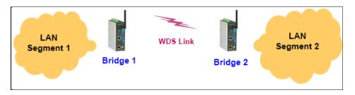
It is a good idea to plan your wireless network by drawing a diagram so that you know how each AWK-4131A is connected to other peer APs or wireless bridges by WDS, and how bridges are connected to other peer bridges by WDS. See the following figure for an example of a network-planning diagram.
