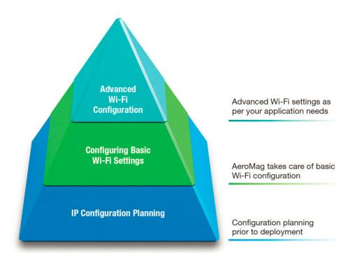
Once you have confirmed the number of APs and their location, using a site-survey tool, and have configured their device names and IP addresses, connect all the APs to the same network using Layer-2 switches. Next, activate the AeroMag function on both the APs and clients.
