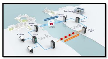
3. **Device Failover:** After covering the communication and frequency failures, in order to provide a single-point-of-failure free wireless network, AeroLink Protection also checks the device status. If the Active node has a power failure, the Backup nodes will automatically resume the wireless communication.
