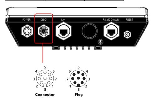
Digital Inputs and Relay-out Pin Assignment (8-pin M12 connector)
