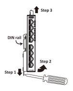
**NOTE** Screws that are used to fix the DIN-rail kit on the SDS-3008 should be securely fastened before mounting on the mounting rail. Please make sure that if you remove the DIN-rail, it must be securely fastened when it is reattached.
