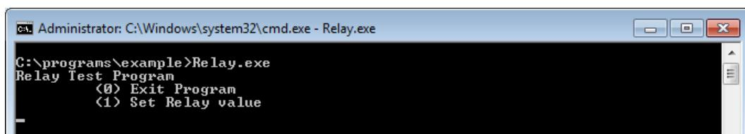
In the example below, the user has selected **1 (Set Relay value)** and is setting the current status of the relay. The value **0** indicates that the relay is currently in normal status as per the jumper setting. The value **1** shown next to the relay entry indicates that the relay is currently in inverse status.
