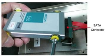
4. Replace the storage drive into the computer and secure it using the four mounting screws you removed in step 1.
