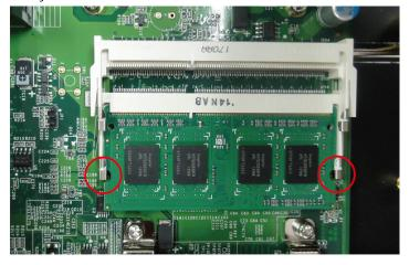
7. Carefully slide the module into the clutch at an angle, and then push downward. Make sure the module has been firmly inserted and is oriented correctly.
