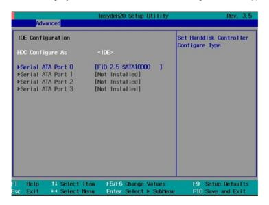
For normal SATA functionality, select AHCI. When this option is selected, AHCI SALP () may be enabled. Four SATA interfaces (0–3)will be highlighted; only the first two SATA ports are enabled by default, with port 0 enabling the removable drive tray on the front panel, and port 1 enabling the drive expansion slot accessed through the bottom panel. The figure below displays the AHCI configuration screen:
