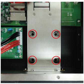
5. When finished, remove the storage tray, and you can see the location of the memory module.
