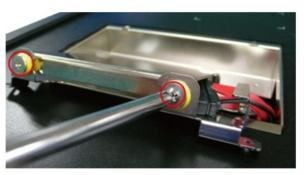
3. Connect the SATA connector to the disk's SATA assembly and then place the hard disk into the mounting tray. Fasten the storage drive to the mounting tray using the side screws you have just removed.
