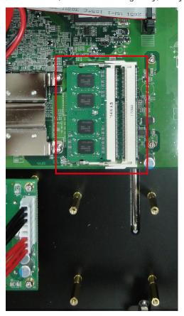
6. There are two clutches on both sides of the module. Click the clutches, and the memory module will pop up. Gently remove the module.
