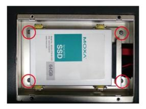
5. Replace and secure the storage drive slot cover to complete the installation
