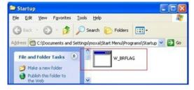
4. The check point function will be enabled each time the system boots up
