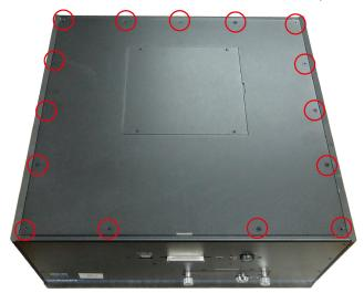
2. Remove the screws on the front panel of the computer, including the screws for the dongle, and remember to take out the removable storage tray on the front panel.
