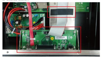
4. Remove the four screws on the removable storage tray.
