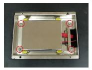
2. Next, remove the four screws located on the sides of the mounting tray and then remove the top cover of the tray.
