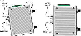
To remove the AWK-3121-M12-RTG from the DIN rail, simply reverse Steps 1 and 2.
