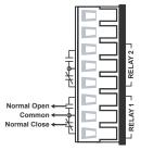
The VPort 451 has two sets of relay output, relay 1 and relay 2, which are located on the 8-pin terminal block connector. Each relay output consists of the 3 contacts of the terminal block on the VPort 451's top panel.
