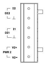
The VPort 451 has two sets of digital inputs, DI1 and DI2. Each DI consists of two contacts of the 6-pin terminal block connector on the VPort's top panel. Top and front views of one of the terminal block connectors are shown here.
