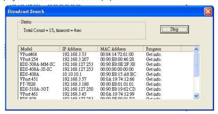
3. When the search has ended, the Model Name, MAC address, and IP address of the EDS Switch and the VPort will be listed in the Utility window.
