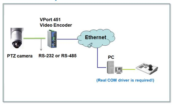
**NOTE** The PTZ control protocol is not standardized. To use a particular PTZ control protocol, the video server must support the driver for that protocol. Currently, the VPort 451 supports PTZ control protocol drivers for:
