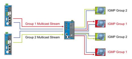
NOTE The VPort 451 is the source that delivers the multicast video stream. To benefit from the Multicast protocol, the gateway or network switch should support the multicast filtering function (such as IGMP Snooping) so that the multicast stream is delivered correctly and precisely. To learn more about IGMP Snooping, refer to the Moxa EtherDeviceTM series Industrial Ethernet Switch user's manual.
