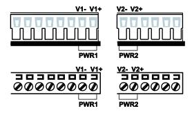
**STEP 1:** Insert the negative/positive DC or AC wires into the V-/V+ terminals.
