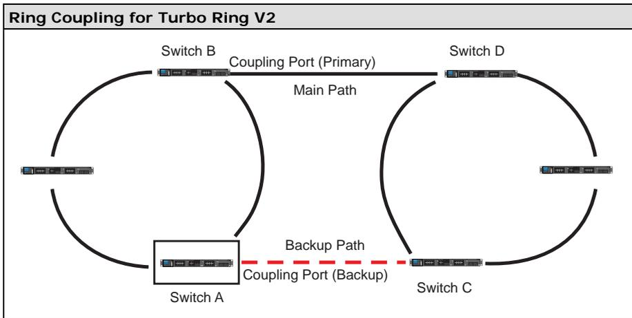
Note that the ring coupling settings for a **Turbo Ring V2** are different from a **Turbo Ring**. For Turbo Ring V2, ring coupling is enabled by configuring the **Coupling Port (Primary)** on Switch B and the **Coupling Port (Backup)** on Switch A only. You do not need to set up a coupling control port, so **Turbo Ring V2** does not require a coupling control line.
