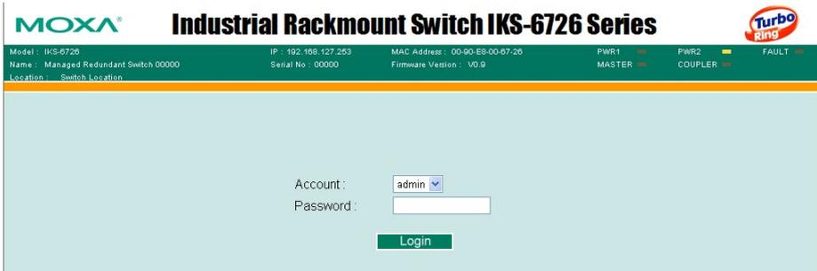
**NOTE** By default, no password is assigned to the IKS-6726's web, serial, and Telnet consoles.
