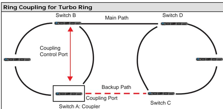
To configure the ring coupling for a **Turbo Ring**, select two IKS series Ethernet switches (e.g., Switch A and B in the above figure) in the ring, and another two IKS series Ethernet switches in the adjacent ring (e.g., Switch C and D).
