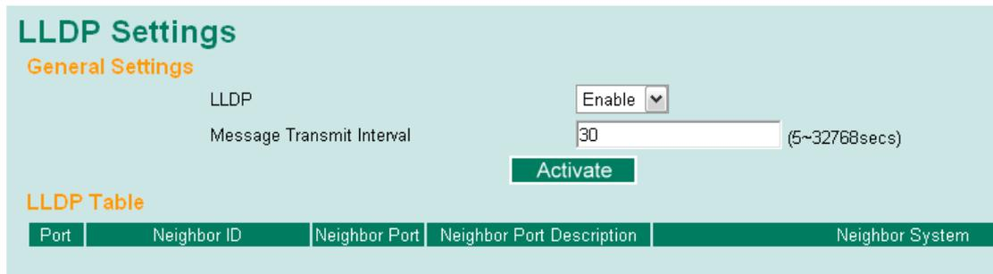
From the switch's web interface, users have the option of either enabling or disabling LLDP, as well as setting the LLDP transmit interval (as shown in the figure below). In addition, users are able to view each switch's neighbor-list, which is reported by its network neighbors. Most importantly, enabling the LLDP function allows Moxa's MXview to automatically display the network's topology and system setup details, such as VLAN and Trunking, for the entire network.
