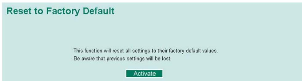
This function provides users with a quick way of restoring the IKS-6726's configuration to factory defaults. This function is available in the serial, Telnet, and web consoles.
