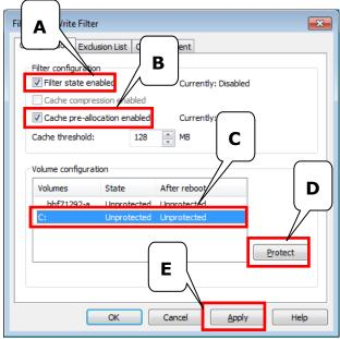
**Cache pre-allocation** sets the memory space available for the overlay cache at the system's start, instead of adjusting it as needed. It cannot be used with cache compression.
