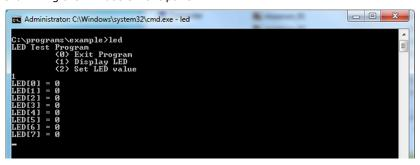
You may now run LED.exe again, but this time select 2. At the next prompt, enter the ID number (0 to 7) of an LED to activate it. When prompted enter either 1 (to turn it on), or 0 (to turn it off). The LEDs on the main DA-683 panel correspond to 0 through 3; 4 and 5 correspond to those on the first module; and 6 and 7 to those on the second.
