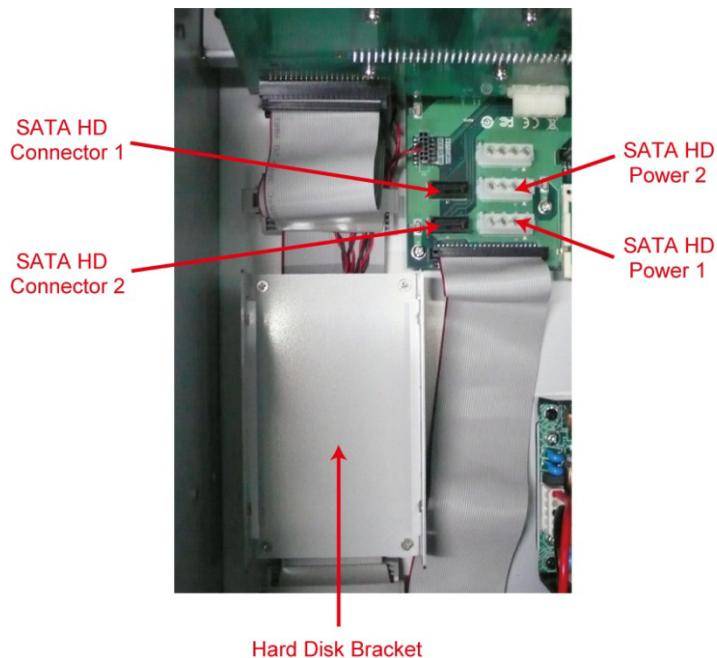
3. Remove the four screws on each corner and remove the hard disk bracket.
