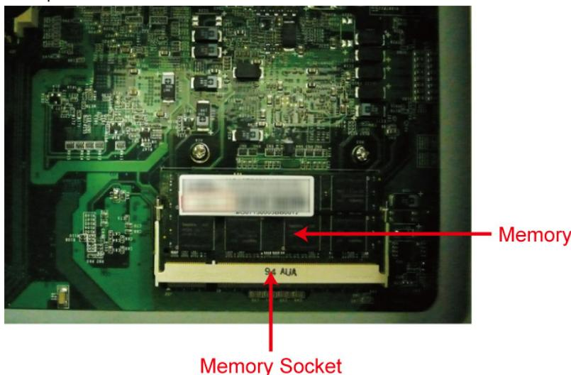
3. There are two clutches on both sides of the module. Click the clutches, and the memory module will pop up. Gently remove the module.
