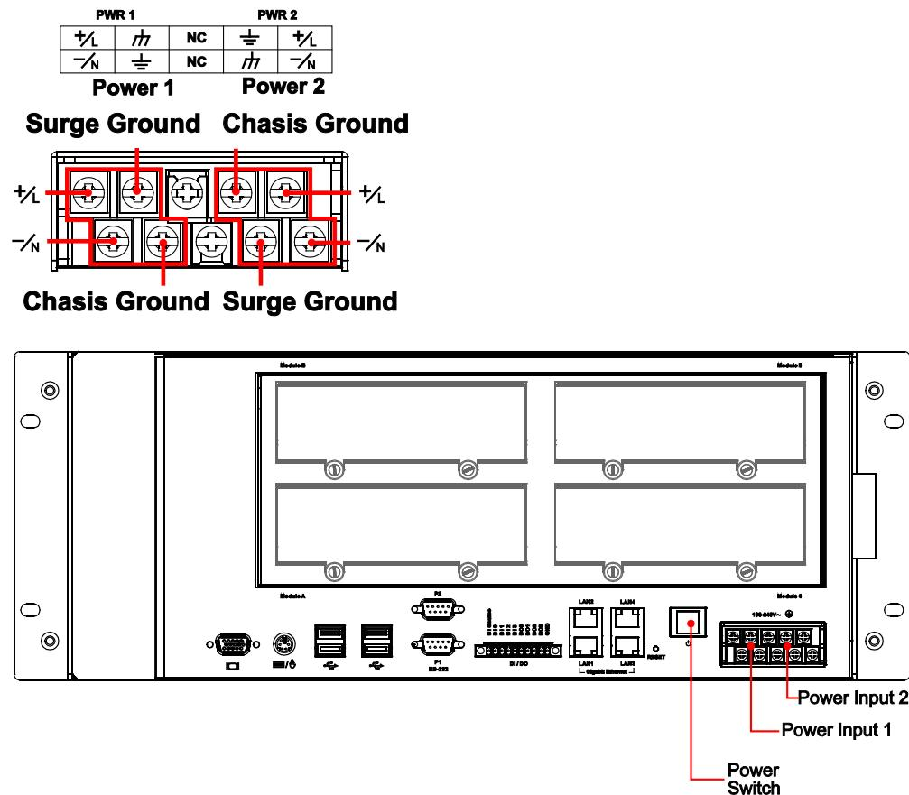
If the power is being properly supplied, the Power LED will light up first, and then the Storage LED will start blinking when the Flash Disk Module is accessed during boot up. It takes about 30 to 60 seconds for the operating system to boot up. If Power 1 or Power 2 is not functioning, the Power 1/2 Fail LED will light up. If this happens, check the power inputs.
