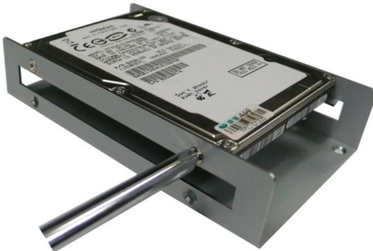
5. Next, install the SATA hard disk and hard disk bracket back into the DA-710. Connect the SATA disk cable and power cable to the SATA hard disk. The DA-710 also offers an IDE connector that can be used to connect to an IDE-based hard disk. However, the IDE connector is being occupied by the DOM. To install an IDE hard disk, remove the DOM first, and then install the hard disk. When finished, connect the disk cable to the IDE connector.
