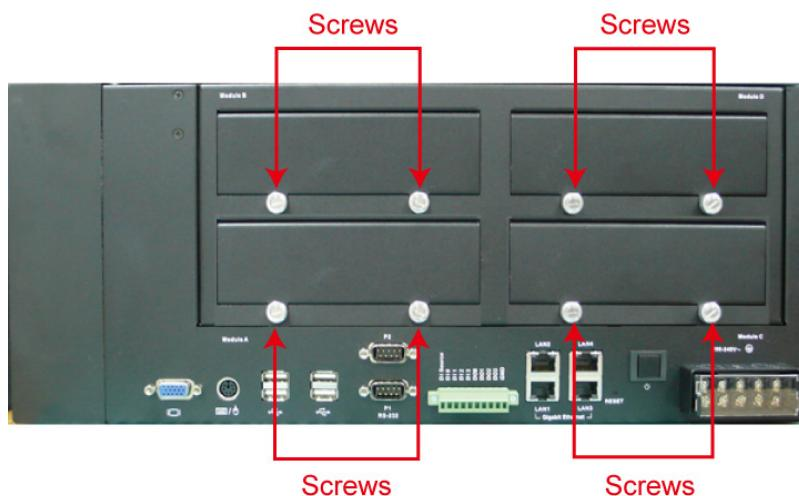
3. Carefully insert or remove the expansion module by pushing or pulling on the two screws at the same time. By pushing or pulling on the two screws evenly, you can ensure that the board is inserted or removed without being damaged.
