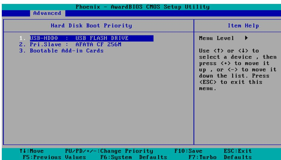
5. Press "+" to move it up to the first priority, and press "Esc" to exit the setup menu.
