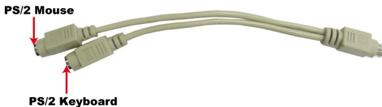
**Note:** Without the Y-type cable, the PS/2 connector on the DA-710 series can only work with a PS/2 keyboard. A PS/2 mouse will not function when directly connected to the PS/2 connector on the DA-710 series.
