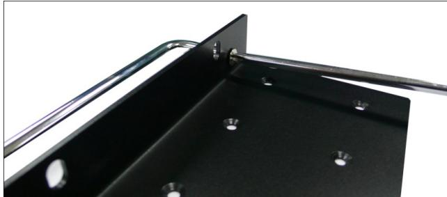
**Step 3: Attaching the rackmount support to the DA-710.**
