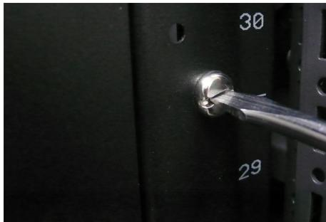
**Note that four screws are required to attach the DA-710 to the rack. Use two screws on each side.**
