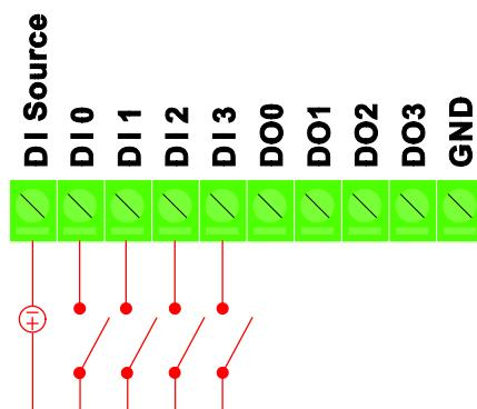
**Note: If you are using wet contacts, you must connect "DI Source" to power.**
