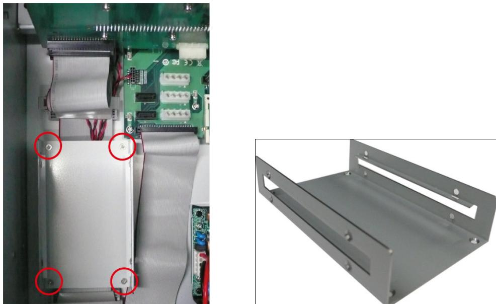
4. Install the SATA hard disk in the hard disk bracket. One bracket can hold up to 2 hard disks; you may use either the upper or lower layer on the bracket to install the hard disk. Fasten the two screws on each side of the bracket.
