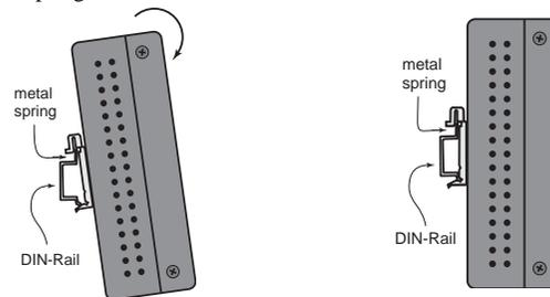
To remove UC-7408 from the DIN-Rail, simply reverse Steps 1 and 2 above.
