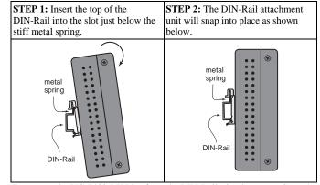
To remove the UC-7402-LX Plus from the DIN-Rail, simply reverse Steps 1 and 2 above.
