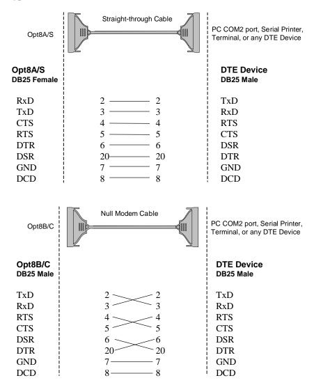
Type 1: To connect Smartio C168 Series to a DTE device.
