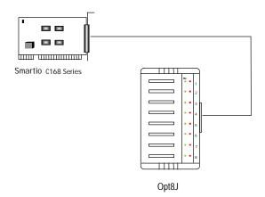
Opt8J is the RS-422/485 connection box with 8 port female DB25 connectors for MOXA 8 port boards, including the Smartio C168 Series. There are 8-DIP switches on the side of the Opt8J. Each switch controls the communication mode (RS-422 or RS-485) of each port, respectively.
