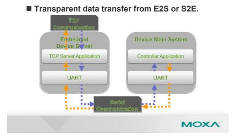
The embedded device server transparently transfers the data from E2S (Ethernet to Serial) or S2E.
