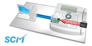
The MiiNePort E1/E2-SDK's SCM (Serial Command Mode) allows the module's parameters to be retrieved or configured through the serial port, rather than over the network. This is done using specially parsed commands sent to the module through the serial port.
