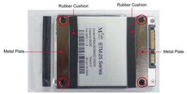
5. The storage drive may now be settled into the expansion slot. Connect the SATA cable first, and then push the drive into the slot to complete the installation. The foam cushions should give the storage drive a snug fit, but if they do not additional shims may be crafted using appropriate, non-volatile materials (paper, etc).
