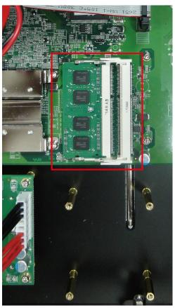
4. There are two clutches, one on either side of the module. Click the clutches to release the card, and the memory module will pop up. Gently remove the module.
