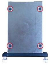
4. Place the drive into the tray and secure it in place using the four screws you have just removed. When finished, insert the tray into the computer and fasten the tray in place using the two thumbscrews on the front panel. Finally, complete the installation by turning the key leftwards to lock the tray into place.
