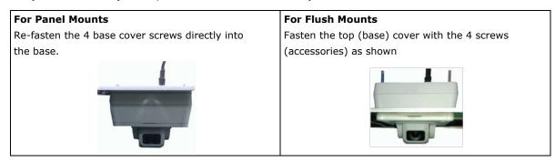
**NOTE** For flush mounts, the 4 top (base) cover screws will fix the VPort 16-M12's top cover to a ceiling panel of 5 mm thickness, maximum. If the standard M4 screws are inadequate, customers may contact their Moxa sales rep to order longer screws.
