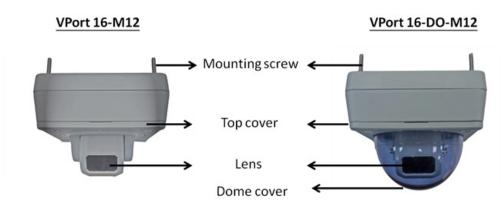
Mounting screw: there are four nylock M4 screws for mounting the VPort 16-M12 on walls or ceilings, giving an external length of about 20mm. These 4 mounting screws can be fastened with nuts, gaskets and spring washers, or directly screwed into a pilot hole.
