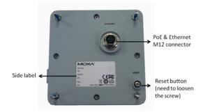
• **PoE & Etherent M12 connector:** A 4-pin M12 A-code connecter for both PoE power supply (Mode A) and Auto MDI/MDI-X Ethernet connections.
