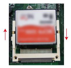
Reverse **steps 9 to 1** to rebuild the unit and complete the system memory and CF card installation.
