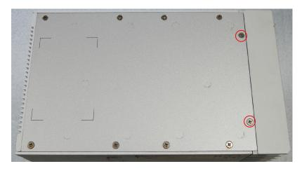
**Step 4:** To get access to the interior of the TC-6110, slide the large heat sink / main interface module in one direction, and the rest of the unit in another.
