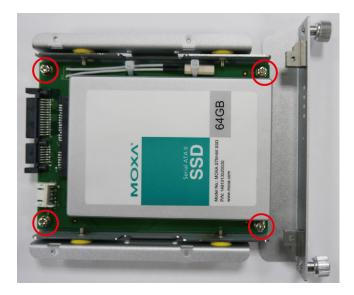
**Step 8:** Connect the power cable and SSD/HDD cable with the main board. Reconnect the data and power interfaces and complete the installation by fastening the drive tray to the main PCB using the six screws.
