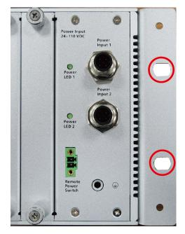
After installing the rack mounting assembly (handles and/or ears), four screws are required to fasten the TC-6110 to a rack.
