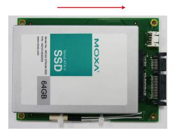
Step 6: Turn back the tray and fasten the drive to the PCB using the holes indicated below.
