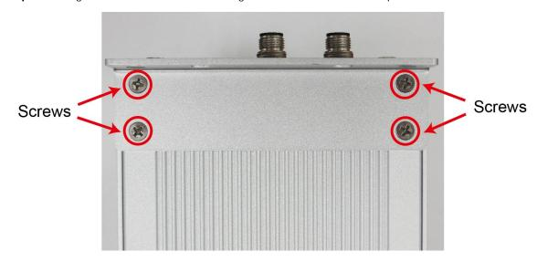
**Step 2:** If you would like to install the handles, use the four screws provided to secure the handles to each of the mounting ears.
