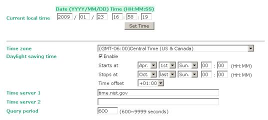
**Current local time** shows the TAP-6226's system time when you open this web page. You can click on the **Set Time** button to activate the update after adjusting the date and time parameters. An "(Updated)" string will appear to indicate that the change is complete. Local time settings will be immediately activated in the system without running Save and Restart.
