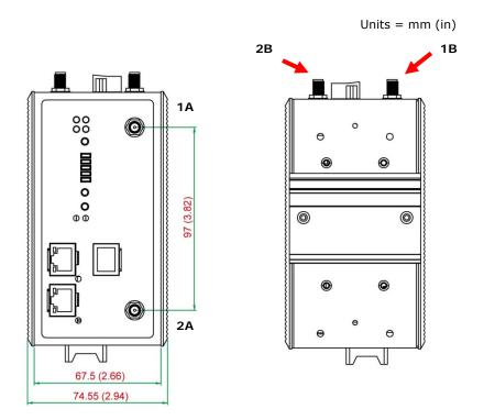
The AWK-5232 provides dual RF technology that meets the 802.11 a/b/g/n standards, giving full 2x2 MIMO. Antennas 1A and 1B are the MIMO antennas associated with RF1, and 2A and 2B are the MIMO antennas associated with RF2.
