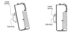
To remove the V2101 from the DIN rail, simply reverse steps 1 and 2.
