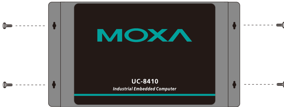
Figure B: UC-8410/8416/8418/8430 Embedded Computer—Wall Mounting Brackets (top view)
